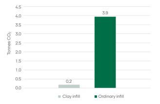
The difference in the carbon footprint using clay infill between half timbering and using ordinary infill consisting of bricks and lime mortar. The calculation is based on the 42 m<sup>2</sup> infill it was necessary to replace at Højgården.
