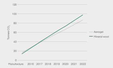
$\uparrow$  CO<sub>2</sub>-emissions using 2 cm aerogel vs. 2 cm mineral wool
