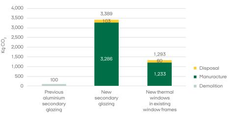
The carbon impact of restoring the windows in Edvard Heiberg's family house. The middle bar is the carbon cost of Realdania By & Byg's attempt to develop special secondary glazing for this and other functionalist buildings.
