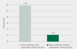
Graph illustrating the issue of "double demolition": Carbon impact of replacing the walkway around Dyrehave Mill, including both demolition of the old balcony and the new walkway, and an alternative LCA including only the new walkway.
