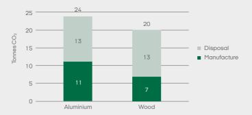
↑ CO<sub>2</sub>-emissions of the full restoration of Poul Henningsen's house using aluminium window frames compared with wood window frames. This grap shows the difference between aluminuum-framed secondary glazing and, as another option, wood frames.
