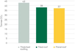
LCA for the whole restoration of Højgården on Sejerø with thatched roof compared with other types of roof. According to the LCA, five tonnes CO<sup>2</sup> more is emitted from a thatched roof than a tiled roof using the generic German EPD for tiled roofs. However, there can be great differences between the different types of roof, and using other, product-specific EPDs could turn things around completely.
