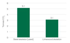
$CO_2$  impact from fitting the steel skeleton in the barn at Højergård to preserve the old walls, compared with a 50% larger timber skeleton.
