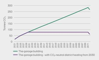
These two graphs show  $CO_2$  savings from insulating the farmhouse and the garage building using wood fibre. Insulation of the garage building will continue to be a  $CO_2$  benefits, while the miller's house will end as a cost, if  $CO_2$ -neutral district heating is fitted in 2030, as there was a certain amount of loft insulation previously.
