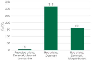
The difference between CO<sub>2</sub> emissions for one tonne of bricks: recycled bricks as used at Hindsgavl and various possible new bricks [including manufacture, disposal and waste treatment].
