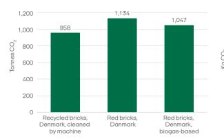
Total CO<sub>2</sub> emissions for the transformation of the farm buildings, as calculated (with recycled bricks), and what they would have been had new bricks been used.
