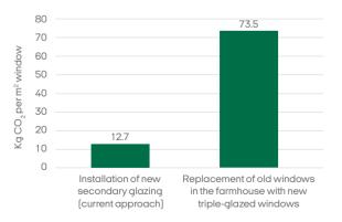
The graph shows the difference in  $CO_2$  emissions from fitting new secondary glazing with wood frames in the farmhouse and the intended replacement of the old windows with new triple-glazed windows, including replacement of the wood frames. The figures shown are per m<sup>2</sup> window area. A gentle transformation of the old barn has worked by giving the building ridge support.
