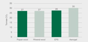
↑ CO₂ emissions from the restoration of Poul Henningsen's house based on a life cycle assessment. The "Aerogel" bar reflects the actual restoration, while the other bars show what the carbon footprint would have been if 2 cm of another insulation material had been fitted.
