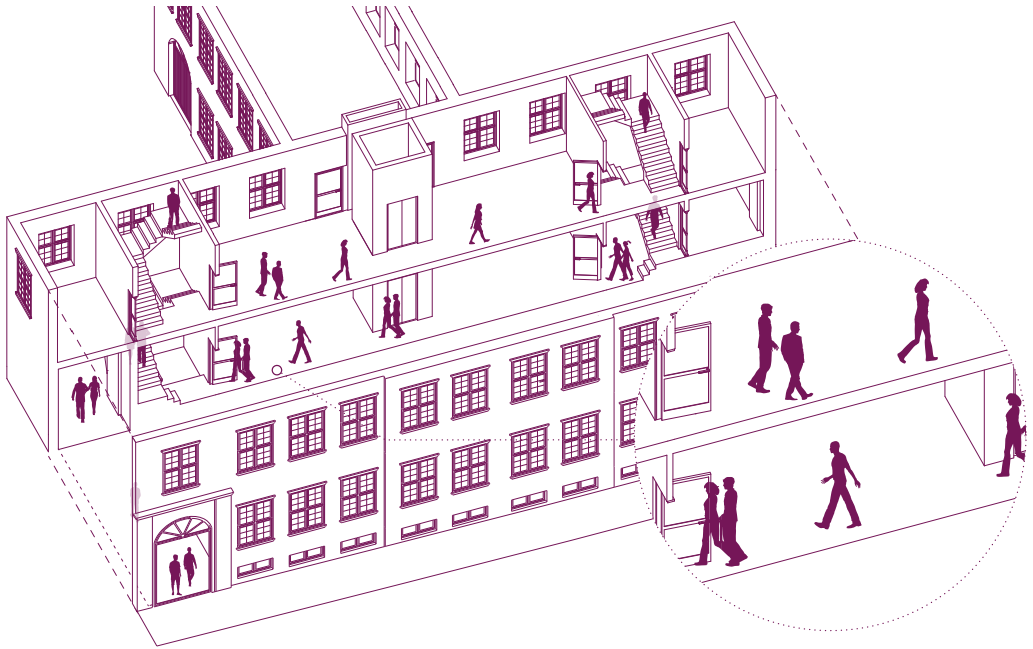
The Danish Association of Architects' building layout makes it possible to establish one-way traffic in corridors and stairways
